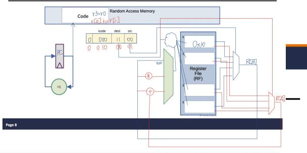
In class, we built a computer that we could program with 1-byte instructions, containing an icode, source, and destination registers. In each cycle, the logic circuits **only** calculated the operation specified by the given icode, which would be later written to a register.
