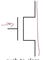
push to close push to connect push to allow current flow
