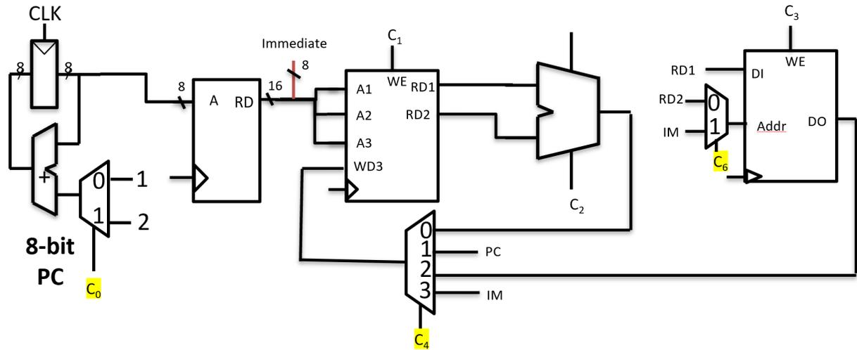
The following three questions ask you to determine the control signals  $C_0$ ,  $C_4$ , and  $C_6$  when  $i\text{code}=6$  and  $b=0$ .
