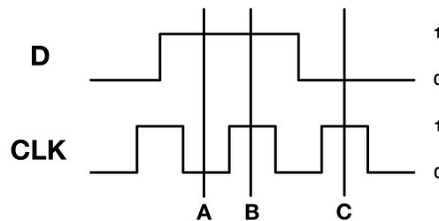
14. (5 points) Given the timing diagram for a positive edge-triggered D flip-flop shown above, what is the value of the output  $Q$  at times A, B, and C?
